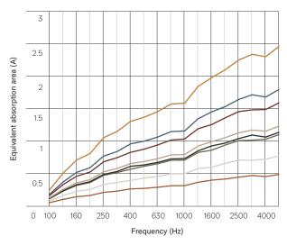
All results are reported in metric sabin - per unit. Equivalent sound absorption area according to ISO 354 measurement of sound absorption in a reverberation room. Average absorption (sabins per unit) calculated at one-third octave bands centred on 250 Hz, 500 Hz, 1000 Hz, and 2000 Hz and rounded to the nearest 0.05.
